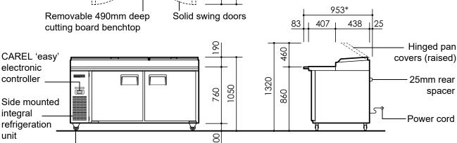
Swivel castors (front locking) or four adjustable legs (100-160mm)
